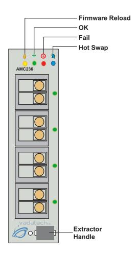
FIGURE 2. AMC235 Front Panel
